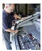
Ron Gremban shows the 18 electric bicycle batteries he added to his converted Toyota Prius. The extra batteries let him store extra power by plugging the car into a wall outlet.
